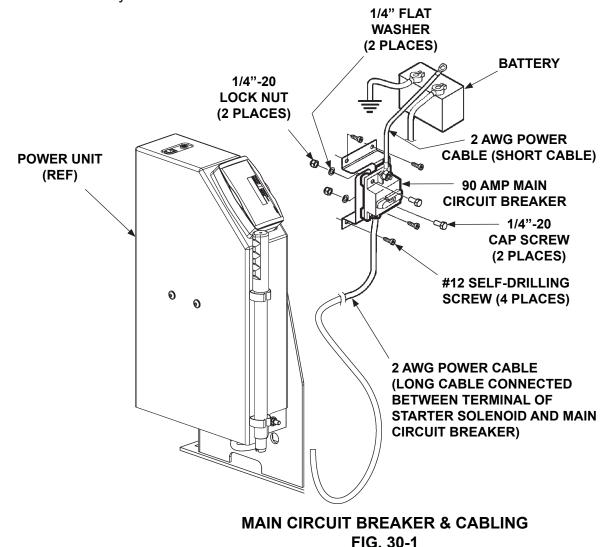
**3.** Lastly, connect one end of long power cable to 90 amp main circuit breaker (FIG. 30-1).
